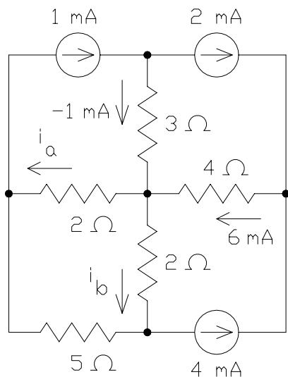
$$i_a + i_b = 6 - 1 = 5 \text{ mA} = 0.005 \text{ A}$$
