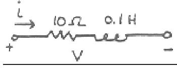
$$\begin{aligned} v &= L \frac{di}{dt} + 10i \\ &= (0.1)(4e^{-t} - 4te^{-t}) + 10(4te^{-t}) \\ &= 0.4e^{-t} + 39.6t e^{-t} \text{ V} \end{aligned}$$
