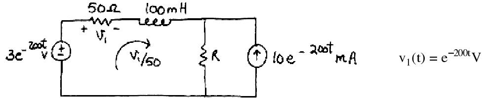
$$\text{KVL a: } -3e^{-200t} + v_1 + .1 \frac{d}{dt} \left( \frac{v_1}{50} \right) + R \left[ \frac{v_1}{50} + .01e^{-200t} \right] = 0$$
