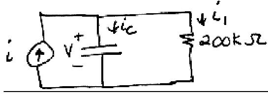
$$i_1 = \frac{v}{200} = \frac{1}{40} (1 - 2e^{-2t}) \text{ mA} = 25 (1 - 2e^{-2t}) \mu\text{A}$$
