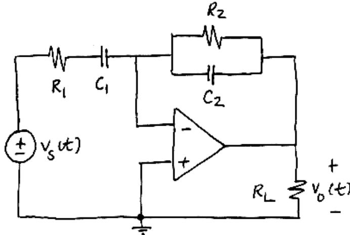
$$H(\omega) = \frac{V_o(\omega)}{V_s(\omega)} = -\frac{R_2 \left| \frac{1}{j\omega C_2} \right|}{R_1 + \frac{1}{j\omega C_1}} = -C_1 R_2 \frac{j\omega}{(1 + j\omega R_1 C_1)(1 + j\omega R_2 C_2)}$$
