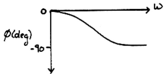
At  $\omega = 0$ ,  $V_i$  and  $V_o$  are in phase. At  $\omega = \infty$ ,  $V_o$  lags  $I_C = V_i / R$  by  $90^\circ$
