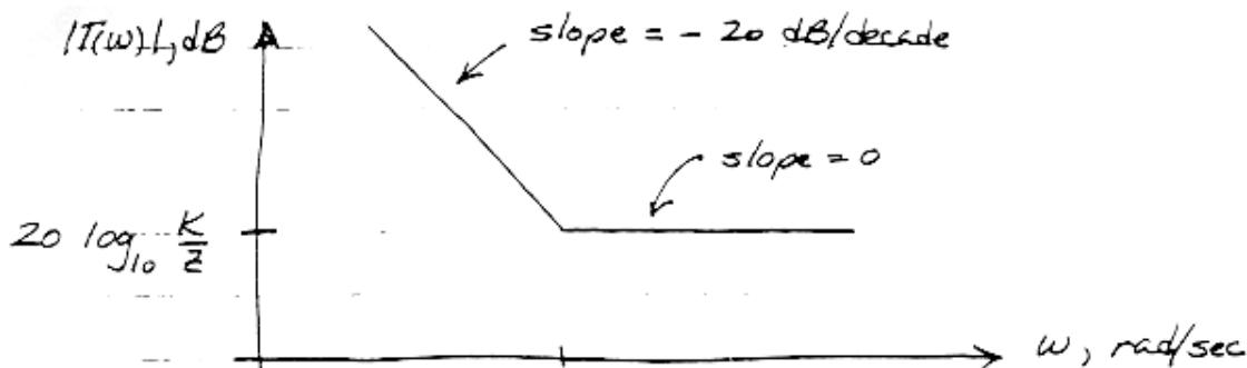
The Bode plot will be within 1% of  $|T(\omega)|$  dB both for  $\omega \ll z$  and for  $\omega \gg z$ . The range when  $\omega \ll z$  is characterized by
