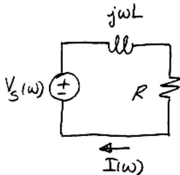
$$H(\omega) = \frac{I(\omega)}{V_s(\omega)} = \frac{1}{R + j\omega L}$$
