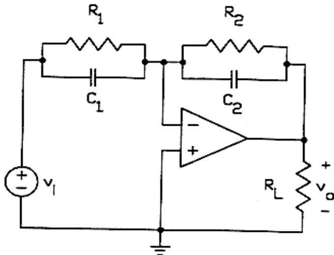
$$H(\omega) = -k \frac{1+j\frac{\omega}{\omega_p}}{1+j\frac{\omega}{\omega_z}}$$
