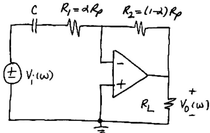
$$H(\omega) = \frac{V_o(\omega)}{V_i(\omega)} = -\frac{R_2}{R_1 + \frac{1}{j\omega C}} = -\frac{j\omega CR_2}{1 + j\omega CR_1} = -\frac{j\omega C(1-\alpha)R_p}{1 + j\omega C\alpha R_p}$$
