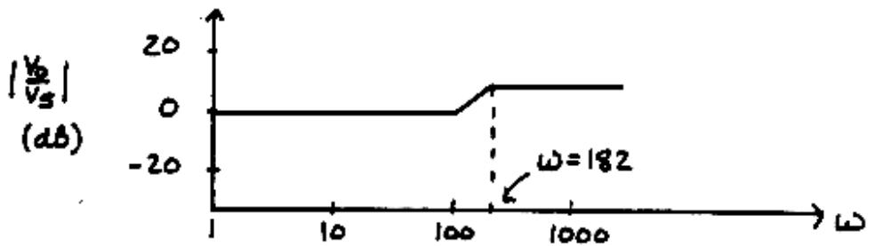
$$C_1 = 0.1 \mu F, \frac{V_o}{V_s} = \frac{1}{2} = \text{constant} \therefore 20 \log \left| \frac{V_o}{V_s} \right| = -3 \text{dB (constant)}$$
