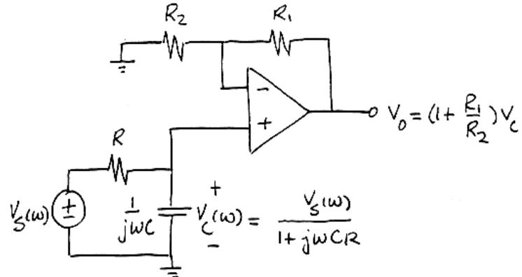
$$V_o(\omega) = \left(1 + \frac{R_1}{R_2}\right) V_c(\omega) = \left(1 + \frac{R_1}{R_2}\right) \frac{1}{1 + j\omega CR} V_s(\omega)$$
