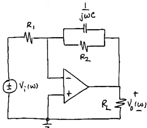
$$\begin{aligned} H(\omega) &= \frac{V_o(\omega)}{V_i(\omega)} \\ &= -\frac{R_2 \parallel \frac{1}{j\omega C}}{R_1} \\ &= \frac{-\left(\frac{R_2}{R_1}\right)}{1+j\omega CR_2} \end{aligned}$$
