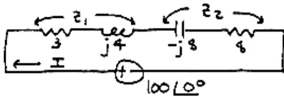
$$(a) \quad Z_1 = 3 + j4 = 5\angle 53.1^\circ \quad Z_2 = 8 - j8 = 8\sqrt{2}\angle -45^\circ$$
