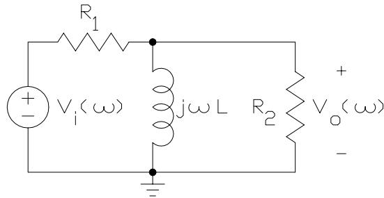
$$\frac{\mathbf{V}_o(\omega)}{\mathbf{V}_i(\omega)} = \frac{\frac{j\omega L R_2}{R_2 + j\omega L}}{R_1 + \frac{j\omega L R_2}{R_2 + j\omega L}} = -\frac{j\omega \frac{L}{R_1}}{1 + j\omega \frac{L}{R_p}}$$
