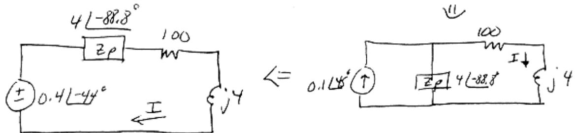
$$I = \frac{0.4 \angle -44^\circ}{-4j + 100 + j4} = 4 \angle -44^\circ \text{ mA; } i(t) = 4 \cos(25000t - 44^\circ) \text{ mA}$$
