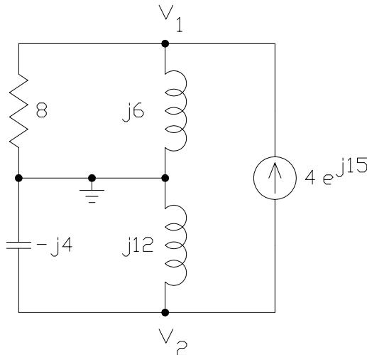
$$\mathbf{V}_1 = 19.2 \angle 68^\circ \text{ and } \mathbf{V}_2 = 24 \angle 105^\circ \text{ V}$$
