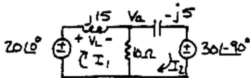
$$\text{KVL at } I_1: j15I_1 + 10(I_1 - I_2) = 20 \\ \Rightarrow (10+j15)I_1 - 10I_2 = 20 \quad (1)$$
