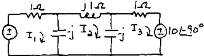
$$\text{Three mesh equations: } (1-j)I_1 + (j)I_2 + 0I_3 = 10$$
