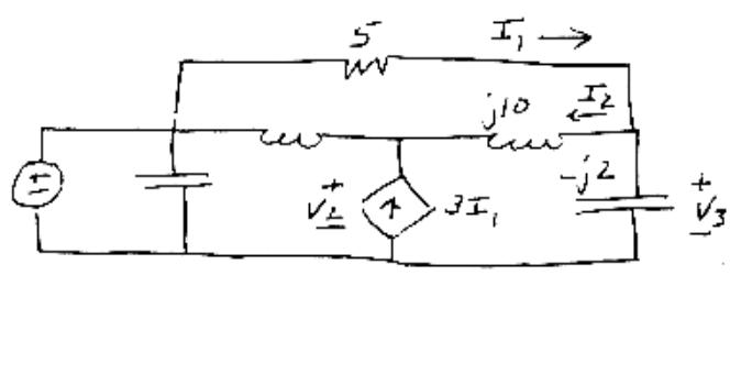
$$V_2 = 0.7571 \angle 66.7^\circ$$
