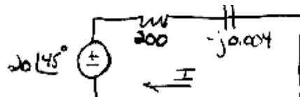
$$I(\omega) = \frac{V}{Z_R + Z_C} = \frac{20 \angle 45^\circ}{200 - j 0.004} = 0.1 \angle 45^\circ$$
