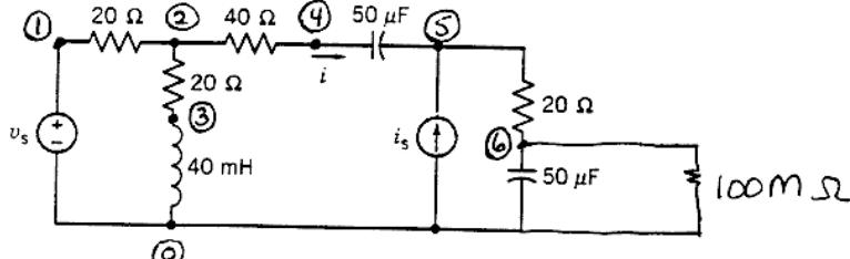
Note: The 100mΩ resistor was added to provide the dc path to ground required by Spice. Since the resistance is so large, it has little effect on the solution calculated.
