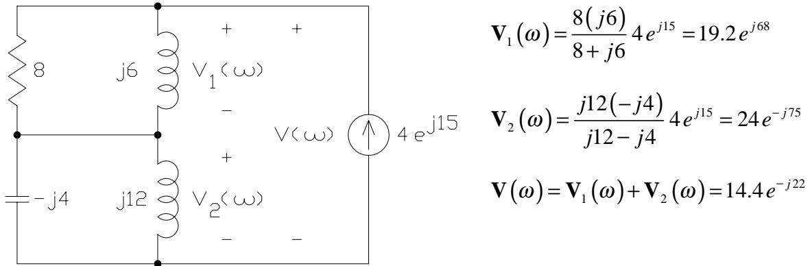
Using superposition:  $v(t) = 3.58 \cos(5t + 47^\circ) + 14.4 \cos(3t - 22^\circ)$
