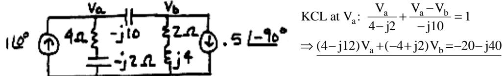
$$\text{KCL at } V_a: \frac{V_a}{4-j2} + \frac{V_a - V_b}{-j10} = 1 \\ \Rightarrow (4-j12)V_a + (-4+j2)V_b = -20-j40$$
