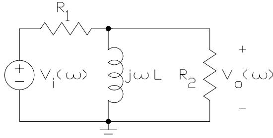
$$\frac{V_o(\omega)}{V_i(\omega)} = \frac{\frac{j\omega L R_2}{R_2 + j\omega L}}{\frac{R_1 + j\omega L R_2}{R_2 + j\omega L}} = -\frac{j\omega \frac{L}{R_1}}{1 + j\omega \frac{L}{R_p}}$$
