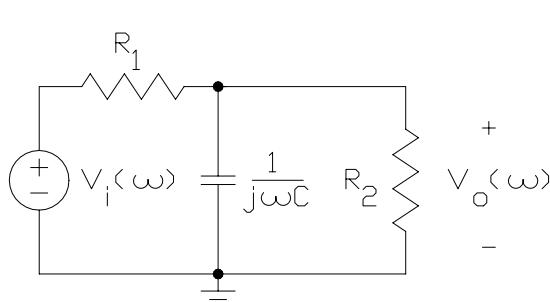
$$R_2 \parallel \frac{1}{j\omega C} = \frac{R_2}{1 + j\omega CR_2}$$
