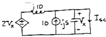
$$V_x = 0 \Rightarrow I_{sc} = 10 \angle 0^\circ \text{ A}$$
