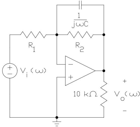
$$R_2 \parallel \frac{1}{j\omega C} = \frac{R_2}{1 + j\omega CR_2}$$
