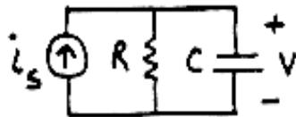
$$\begin{aligned} \text{KCL: } i_s &= v/R + C \frac{dv}{dt} \\ \frac{dv}{dt} + \frac{v}{RC} &= \frac{I_m}{C} \cos \omega t \end{aligned}$$
