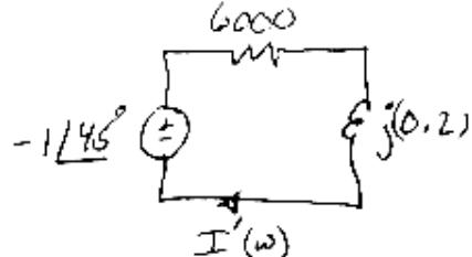
$$I'(\omega) = \frac{-1\angle 45^\circ}{6000+j0.2} = -0.166 \times 10^{-3} \angle 45^\circ$$
