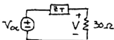
$$V = V_{oc} \left( \frac{30}{30 + Z_T} \right) = -j \frac{300}{9-j} = 33.13 \angle -83.66^\circ \text{ V}$$
