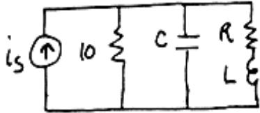
$$\left. \begin{array}{ll} Z_1 = 10 & Y_1 = 1/10 \\ Z_2 = 1/j\omega C & Y_2 = j\omega C \\ Z_3 = R + j\omega L & Y_3 = 1/(R + j\omega L) \end{array} \right\}$$
