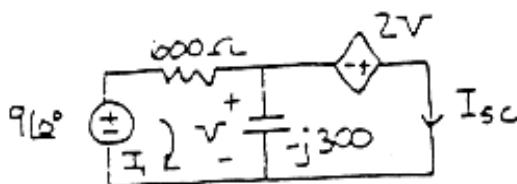
$$\text{KVL loop } I_{sc}: -2V - V = 0 \Rightarrow V = 0$$
