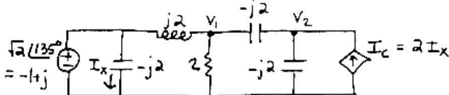
$$\text{node } V_1: \frac{V_1 - (-1+j)}{j2} + \frac{V_1}{2} + \frac{V_1 - V_2}{-j2} = 0 \quad (1)$$
