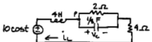
$$\left. \begin{array}{l} \text{So } v_c(0^+) = 5 = A_1 + A_2 + 2 \Rightarrow A_1 + A_2 = 3 \\ \frac{dv_c(0^+)}{dt} = -30 = -2A_1 - 3A_2 + 2 \Rightarrow 2A_1 + 3A_2 = 32 \end{array} \right\} \left. \begin{array}{l} A_1 = -23 \\ A_2 = 26 \end{array} \right.$$
