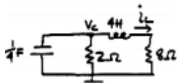
$$\text{KCL at } v_c : \frac{1}{4} \frac{dv_c}{dt} + \frac{v_c}{2} + i_L = 0 \quad (1)$$
