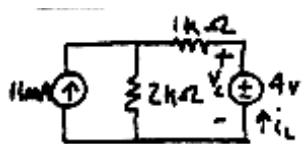
$$v_c(0^-) = 4V = v_c(0^+) \text{ & from KVL: } -4 + i_L + 2(11 + i_L) = 0 \\ \Rightarrow i_L(0^-) = i_L(0^+) = -6 \text{ mA}$$
