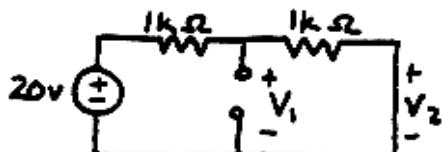
$$v_2(0^-) = 0 = v_2(0^+) \quad \& \quad v_1(0^-) = 10V = v_1(0^+)$$
