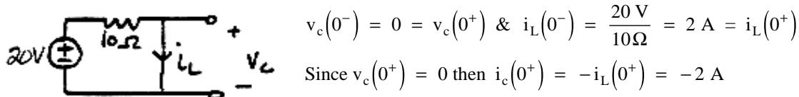
$$v_c(0^-) = 0 = v_c(0^+) \text{ & } i_L(0^-) = \frac{20 \text{ V}}{10 \Omega} = 2 \text{ A} = i_L(0^+)$$
