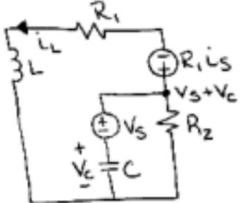
$$\text{KCL: } i_L + C \frac{dv_c}{dt} + \frac{v_s + v_c}{R_2} = 0$$
