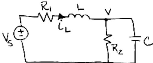
$$\text{KCL: } i_L = \frac{v}{R_2} + C \frac{dv}{dt}$$
