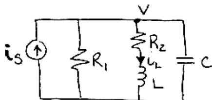
$$\text{KCL: } i_s = \frac{v}{R_1} + i_L + C v$$
