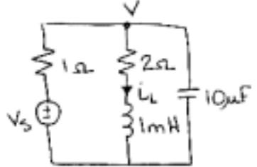
$$\text{KCL: } \frac{v - v_s}{1} + i_L + 10\mu \frac{dv}{dt} = 0 \quad \text{where } \mu = 10^{-6}$$
