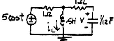
$$\text{KCL at top node: } \left( .5 \frac{di_L}{dt} - 5 \cos t \right) + i_L + \frac{1}{12} \frac{dv}{dt} = 0 \quad (1)$$
