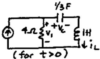
$$\text{KVL at right mesh: } v_c + si_L + 4(i_L - 2) = 0 \quad (1)$$
