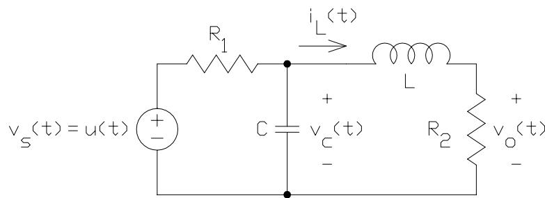
When the circuit reaches steady state after  $t = 0$ , the capacitor acts like an open circuit and the inductor acts like a short circuit. Under these conditions
