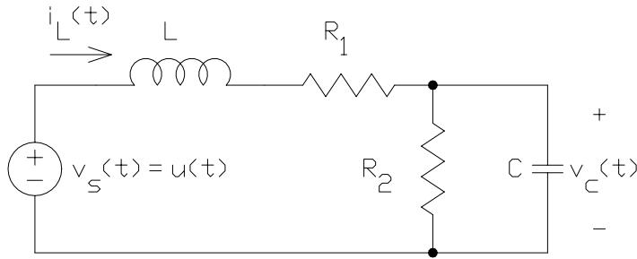
When the circuit reaches steady state after  $t = 0$ , the capacitor acts like an open circuit and the inductor acts like a short circuit. Under these conditions
