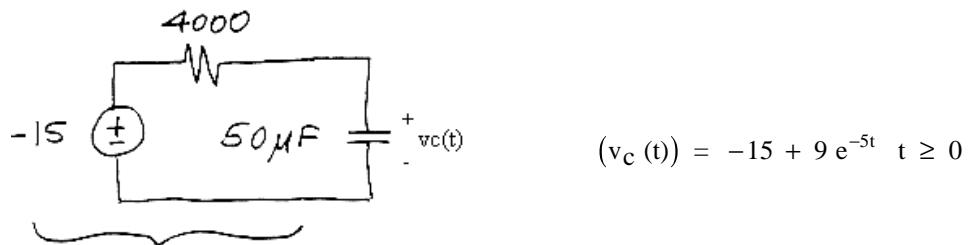
Thévenin equivalent of the circuit connected to the capacitor
