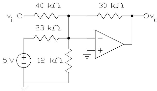
**DP 6-3 (a)**  $12v_i + 6 = 24\left(\frac{1}{2}v_i + \frac{1}{20}(5)\right) \Rightarrow K_4 = 24, K_1 = \frac{1}{2}, \text{ and } K_2 = \frac{1}{20}$ . Take  $R_a = 18$   $k\Omega$  and  $R_b = 1$   $k\Omega$  to get
