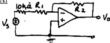
$$\frac{v_o}{v_s} = -\frac{R_2}{R_1 + R_s}$$
