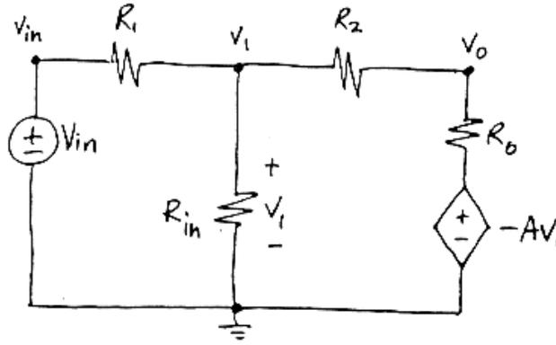
$$\left. \begin{aligned} \frac{v_1 - v_{in}}{R_1} + \frac{v_1}{R_{in}} + \frac{v_1 - v_0}{R_2} &= 0 \\ \frac{v_0 + Av_1}{R_0} + \frac{v_0 - v_1}{R_2} &= 0 \end{aligned} \right\} \Rightarrow \frac{v_0}{v_{in}} = \frac{R_{in}(R_0 - AR_2)}{(R_1 + R_{in})(R_0 + R_2) + R_1 R_{in}(1 + A)}$$
