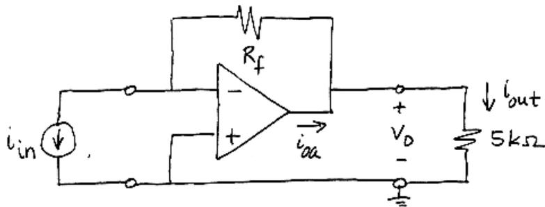
is described by  $v_o = R_f i_{in}$ . Since  $i_{out} = \frac{v_o}{5k\Omega}$
