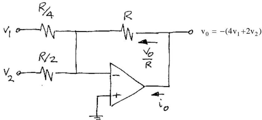
$$|i_0| \leq \frac{4|v_1| + 2|v_2|}{R} \leq \frac{6}{R} < i_{\text{sat}} \quad \text{so } R > \frac{6}{i_{\text{sat}}} = \frac{6}{2 \times 10^{-3}} = 3 \text{ k}\Omega \text{ is required}$$
