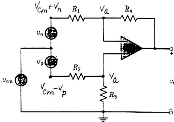
$$v_a = \frac{R_3}{R_2 + R_3}(v_{cm} - v_p)$$
