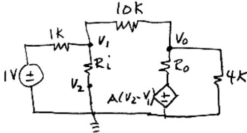
$$A = 10^4, R_i = 200\text{k}\Omega, R_o = 5\text{k}\Omega$$
