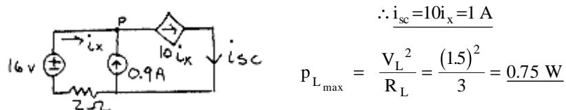
$$\therefore R_T = v_{oc}/i_{sc} = 3\Omega = R_L \quad \text{for max power}$$
