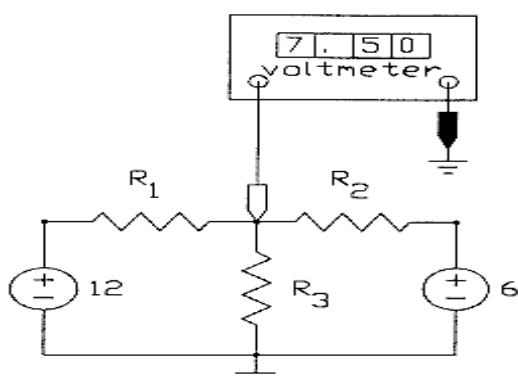
There are only three cases to consider. Suppose  $R_1 = 5\text{k}\Omega$  and  $R_2 = 10\text{k}\Omega$ . Then
