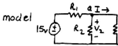
$$\text{KCL at a: } \frac{v_2 - 15}{R_1} + \frac{v_2}{R_2} + I = 0$$
