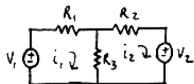
$$\text{mesh } i_1: (R_1 + R_3) i_1 - R_3 i_2 - v_1 = 0 \quad (1)$$
