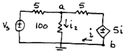
$$\begin{aligned} v_{ab} &= 5i + 5i = 10i \\ \therefore P_{\text{motor}} &= (v_{ab})i = 10i^2 = 150 \\ \Rightarrow i &= \sqrt{15} \text{ A} \end{aligned}$$
