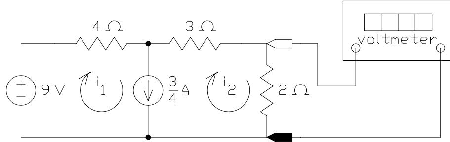
$$\text{Express the current source current in terms of the mesh currents: } \frac{3}{4} = i_1 - i_2 \Rightarrow i_1 = \frac{3}{4} + i_2.$$
