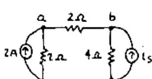
$$\text{KCL at node } a : v_a \left( \frac{1}{2} + \frac{1}{2} \right) - \frac{1}{2} v_b - 2 = 0 \quad (1)$$
