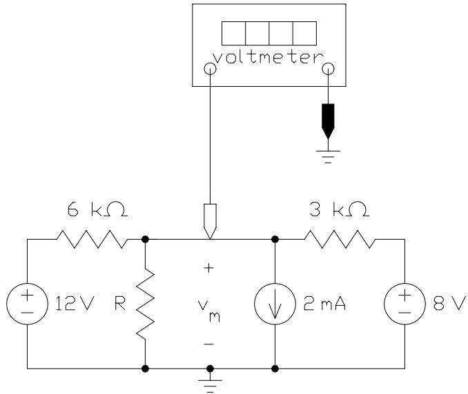
Write a node equation at the node at which the node voltage is measured.
