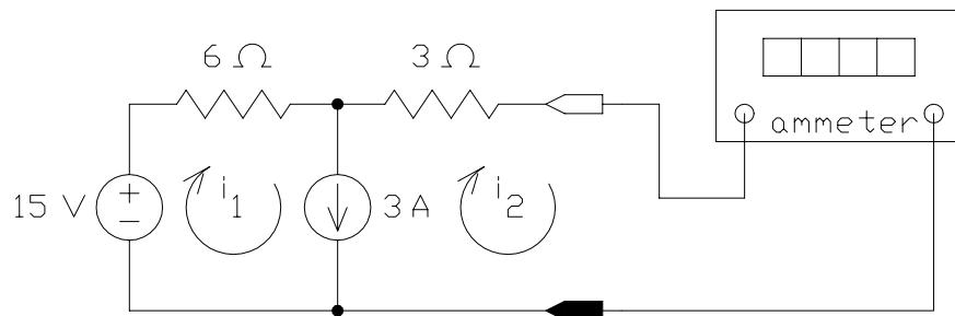
$$\text{Express the current source current in terms of the mesh currents: } 3 = i_1 - i_2 \Rightarrow i_1 = 3 + i_2.$$
