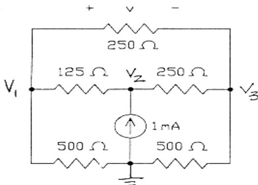
$$\frac{v_1}{500} + \frac{v_1 - v_2}{125} + \frac{v_1 - v_3}{250} = 0$$
