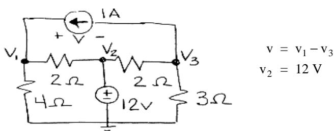
$$\text{KCL at } v_1: \frac{v_1}{4} + \frac{v_1 - v_2}{2} - 1 = 0$$
