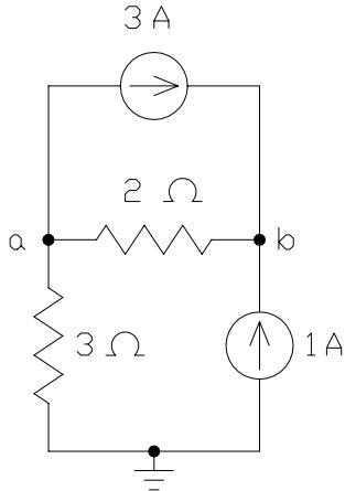
$$\text{KCL at a: } \frac{v_a}{3} + \frac{v_a - v_b}{2} + 3 = 0 \Rightarrow 5v_a - 3v_b = -18$$
