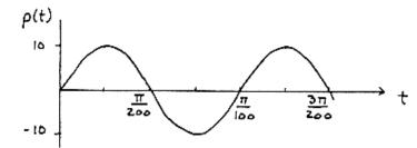
b) power absorbed for  $\frac{2n\pi}{200} < t < \frac{(2n+1)\pi}{200}$  n = 0,1,2... power delivered for  $\frac{(2n-1)\pi}{200} < t < \frac{2n\pi}{200}$  n = 1,2,3...
