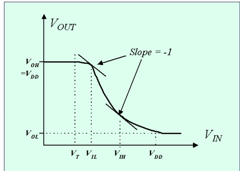
Good:  $V_{OH} = V_{DD}$
