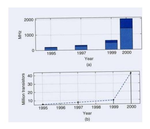
(a) Range of CPU speeds in MHz, (b) Number of transistors in each of the above chips
