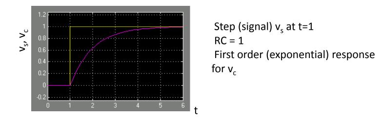
Note, we could also have considered the voltage across the resistor or the current as signals
