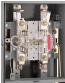
200 A Ringless-Type Meter Socket, 5-Jaw with Lever Type Bypass Shown with Lexan Shield over Line and Load Meter Jaws
