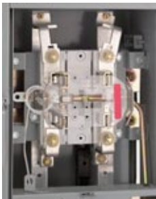
400 A Ringless-Type Meter Socket, 5-Jaw with Lever Type Bypass Shown with Lexan Shield over Line and Load Meter Jaws
