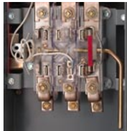
400 A Ringless-Type Meter Socket, 7-Jaw with Lever Type Bypass Shown with Lexan Shield over Line and Load Meter Jaws
