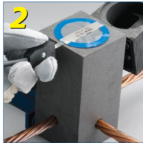
Attach control unit termination clip to ignition strip
