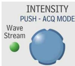
The **INTENSITY** knob adjusts the brightness of your trace. Pushing the button toggles between WaveStream fast-viewing mode (indicator lamp on) and real-time mode (lamp off).
