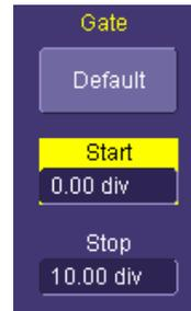
Sometimes you might want to have a parameter measurement on a specific portion of your signal, and ignore all other portions. When this is the case, you can use Measure **Gate**. Measure **Gate** is controlled in the Measure dialog, and is set in grid divisions.
