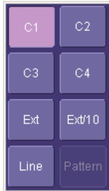
**C1** through **C4** are abbreviations for Channel 1 through Channel 4.
