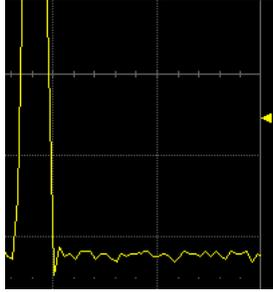
The trigger level Indicator is a color-coded triangle that is positioned vertically on the grid.
