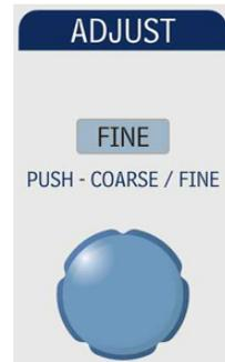
To set the gate, touch the **Start** field to highlight the control yellow, and then use the adjust knob to adjust the location of the start gate. Repeat for the **Stop** gate. Measure gates will remain on the display as long as the **Start** gate is not equal to 0 divisions, and the **Stop** gate is not equal to 10 divisions.
