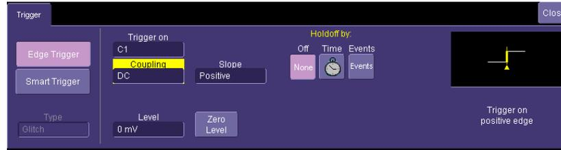
Make sure that “**Edge Trigger**” is highlighted, and not “**SMART Trigger**”
