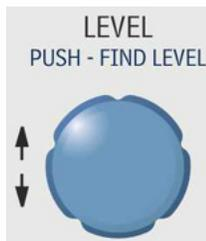
To change trigger level, use the front panel knob in the Trigger Control area. Rotate the knob to adjust, or push to set to 50% of the signal level.
