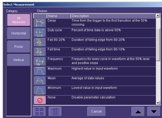
Touch any of the icons to select the measurement that you desire. Scroll down through the list using the slider bar on the right side of the pop-up menu.
