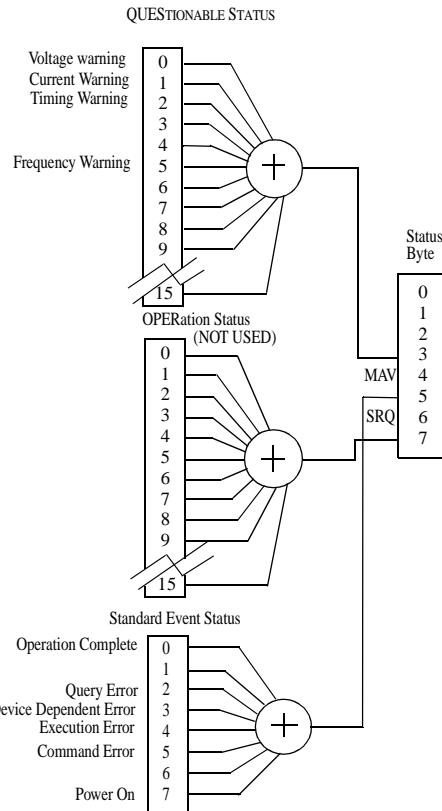
The instrument has a status reporting system conforming to IEEE 488.2 and SCPI. The figure above shows the status groups available in the instrument.
