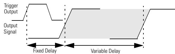
The specified and displayed value is that obtained with the fastest leading edge. Pulse delay has two components, a fixed delay from trigger output to output signal and a variable delay with respect to the trigger output.
