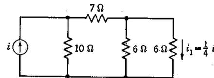
Fig. 3-24 Current gain in a resistive network.
