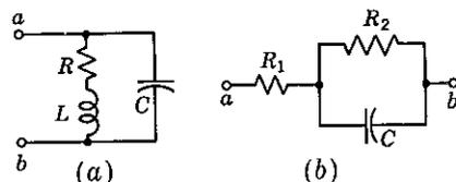
Fig. 3-3 Series-parallel connection of elements.
