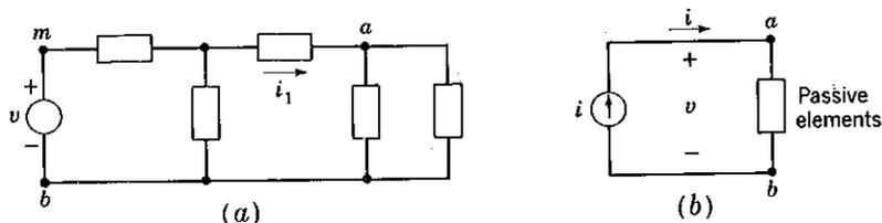
Fig. 3-22 (a) The network functions that relate  $v_{ab}$  or  $i_1$  to  $v_{mb}$  is a transfer function. (b) Driving-point immittance relates  $v$  and  $i$ .
