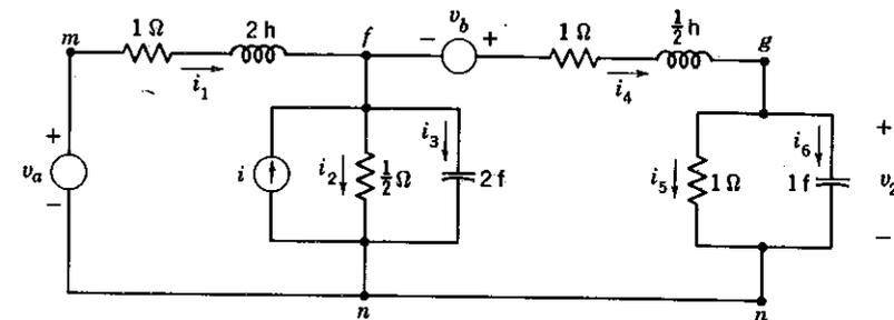
Fig. 3-26 Circuit with three source functions used in Example 3-10.
