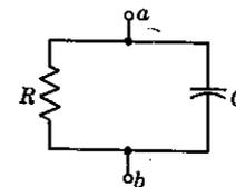
Fig. 3-2 Parallel connection of two elements.
