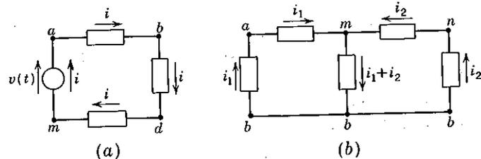
Fig. 3-6 (a) Network consisting of one loop. (b) A two-mesh network.
