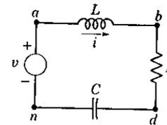
Fig. 3-18 A series R-L-C circuit excited by an ideal voltage source.
