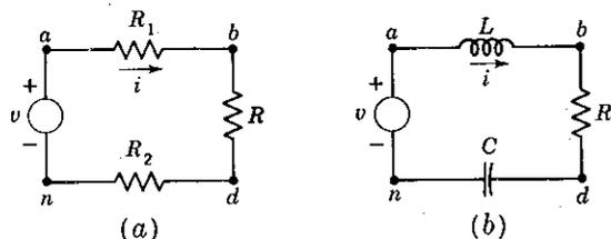
Fig. 3-20 (a) A resistive circuit. (b) An  $R$ - $L$ - $C$  circuit with the same number of elements as the circuit of (a).
