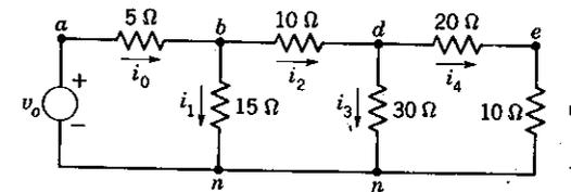
Fig. 3-9 Resistive ladder network.
