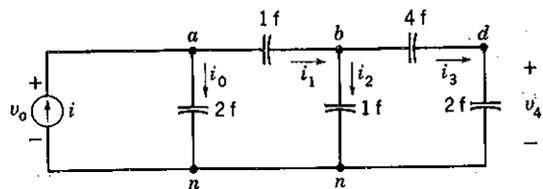
Fig. 3-10 Capacitive ladder network.
