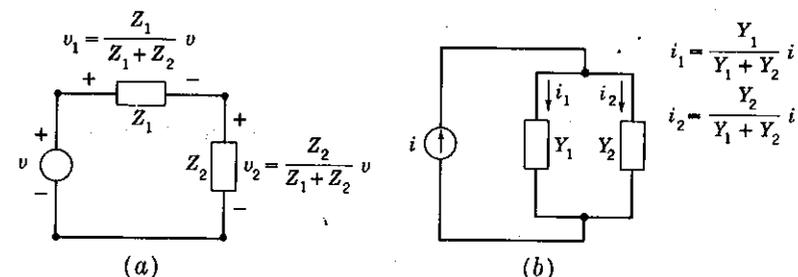
Fig. 3-23 (a) Voltage division for operational impedances. (b) Current division for operational admittances.
