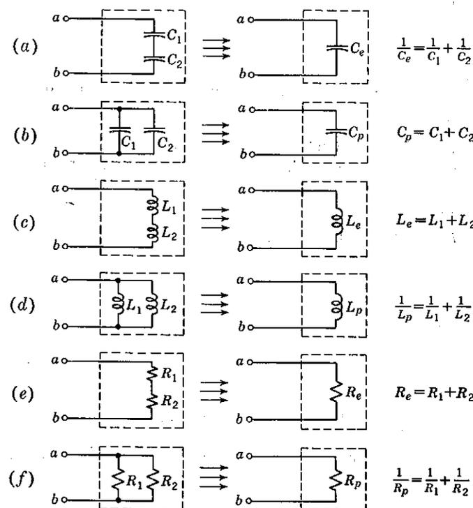
Fig. 3-11 Equivalent elements.
