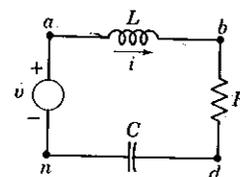
Fig. 3-7 A series R-L-C circuit excited by an ideal voltage source.
