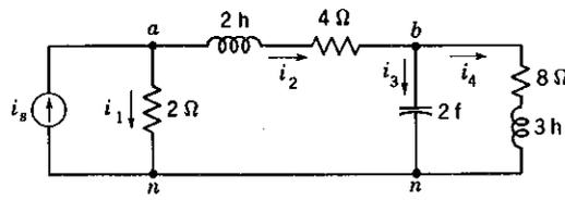
Fig. 3-21 Ladder network analyzed in Example 3-8.
