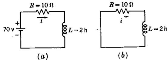
Fig. 3-27 (a) An R-L circuit with a source.
