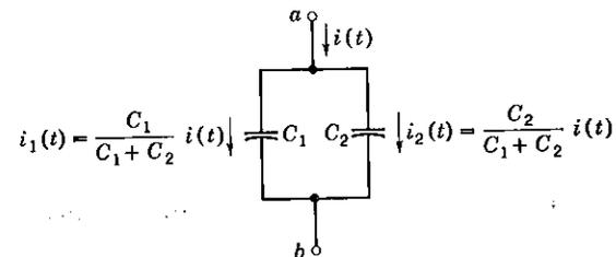
Fig. 3-17 Current division in parallel capacitances.
