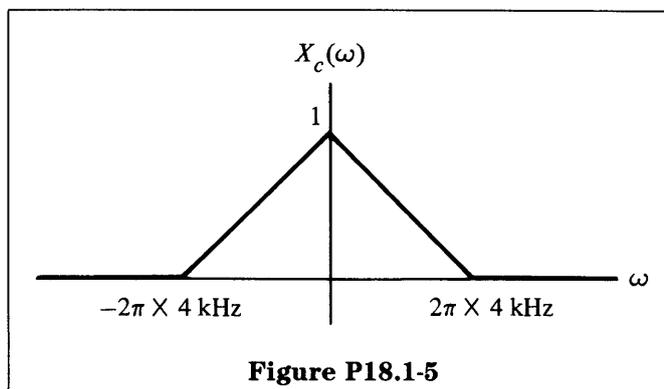
The sampling frequency is 8 kHz. Sketch accurately the following transforms.
