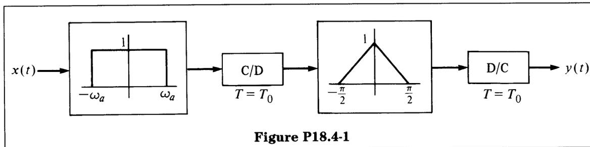
Find, in terms of  $\omega_c$ , the value of the sampling period  $T_0$  and the corresponding value  $\omega_a$  such that the total continuous-time filter has the frequency response shown in Figure P18.4-2.
