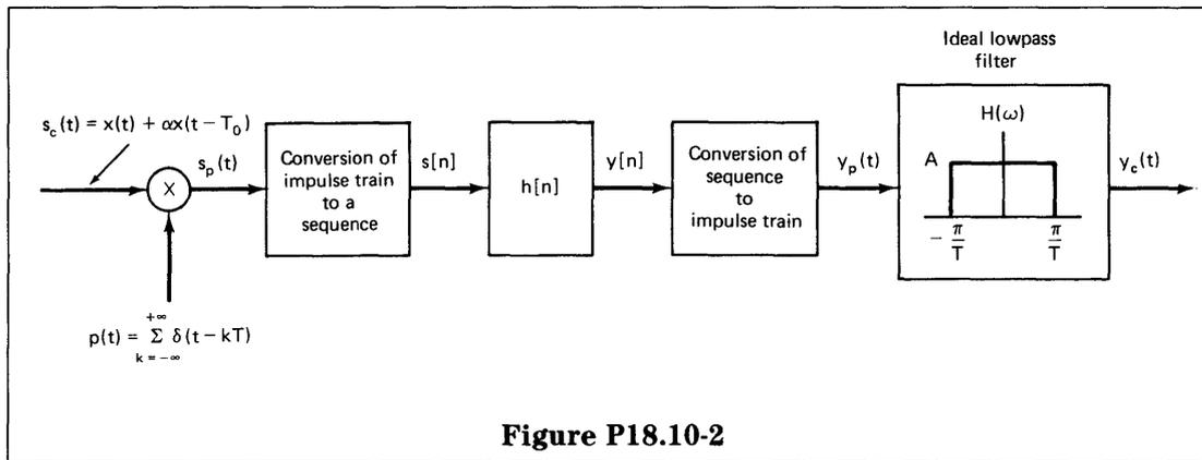
Assume that  $x(t)$  is bandlimited, i.e.,  $X(\omega) = 0$  for  $|\omega| > \omega_M$ , and that  $|\alpha| < 1$ .
