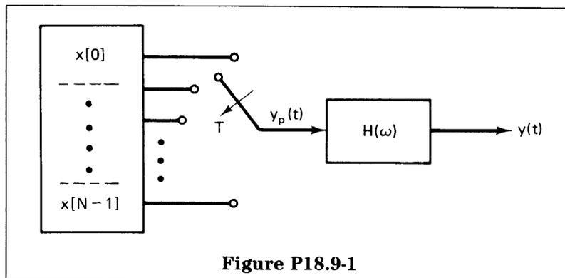
The parameter  $\omega_c$  is to be determined such that  $y(t)$  is a continuous-time cosine signal in the desired frequency band.
