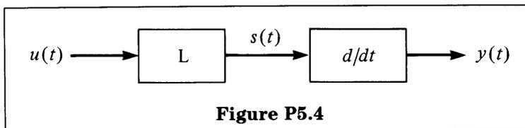
Using the fact that the overall response of LTI systems in cascade is independent of the order in which they are cascaded, show that the impulse response of system L is the derivative of its step response, i.e.,
