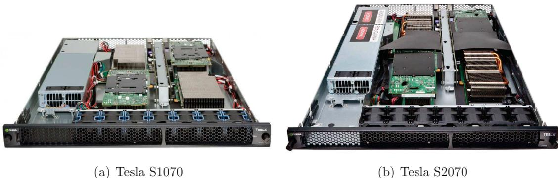
**Figure 1.6.** NVIDIA Tesla S1070 [5] and Tesla S2070 [6] includes four GT200 and GF100 GPUs respectively in the single 1U rack mount
