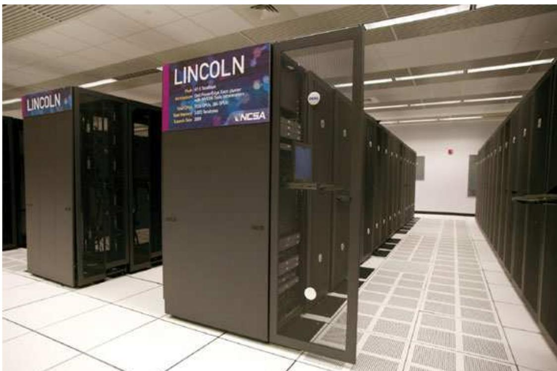
**Figure 1.8.** Lincoln Teragrid/XSEDE GPU cluster with 384 Tesla 10 series GPUs (from [7])
