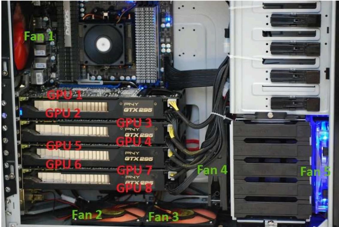
**Figure 1.7.** Orion in-house supercomputer with AMD quad-core Phenom II X4 CPU and four GTX 295 cards
