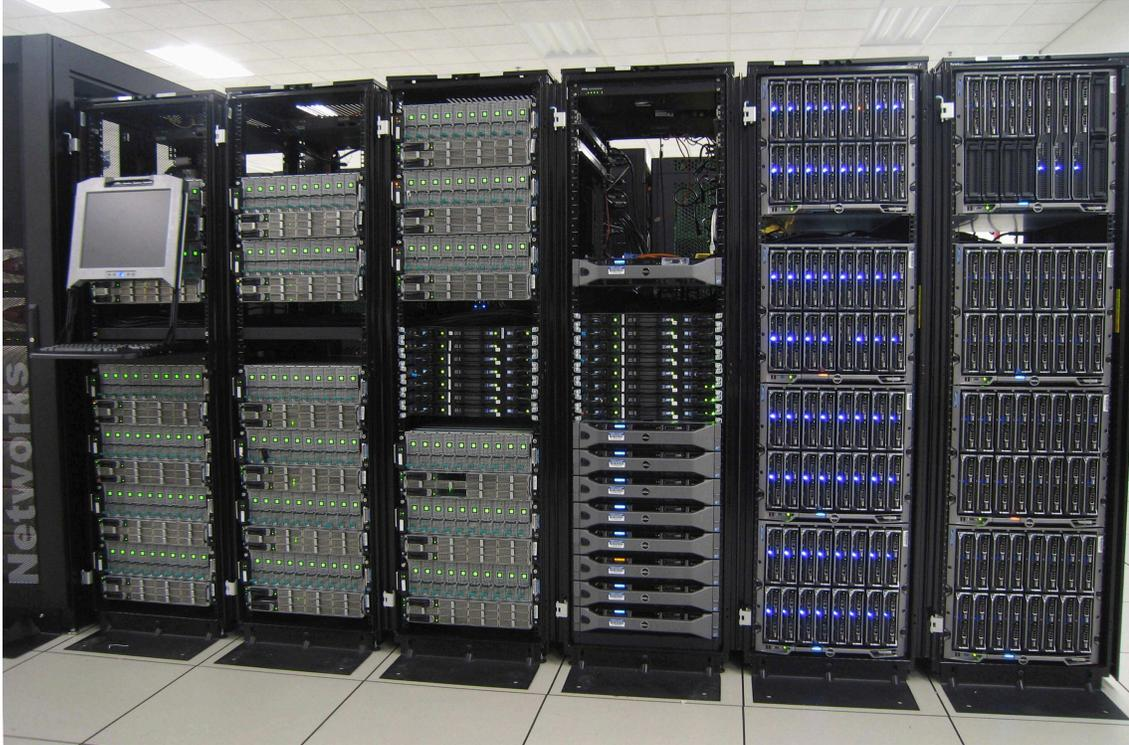
**Figure 1.9.** Forge Teragrid/XSEDE GPU cluster with 288 Tesla 20 series GPUs (from [8])
