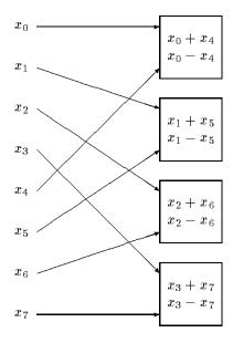
Figure 1: Omega network computing  $(I_4 \otimes F_2)L_4^8$
