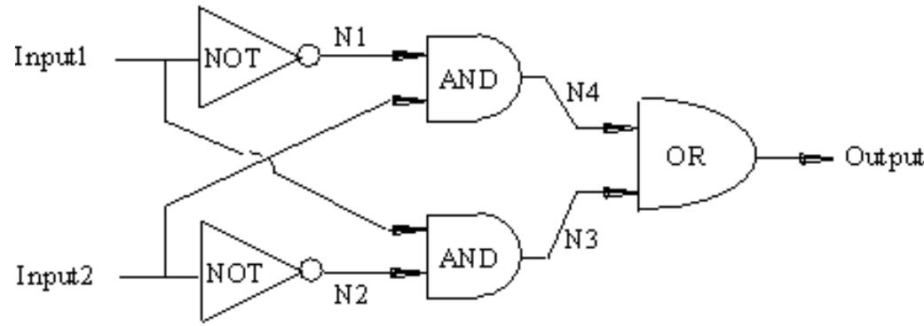
construct an exclusive OR circuit from AND, OR, and NOT circuits, and then check its operation
